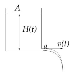
From energy conservation  $v = \sqrt{2gH}$ , from incompressibility AH' = -eav, where e is the efflux coefficient.
